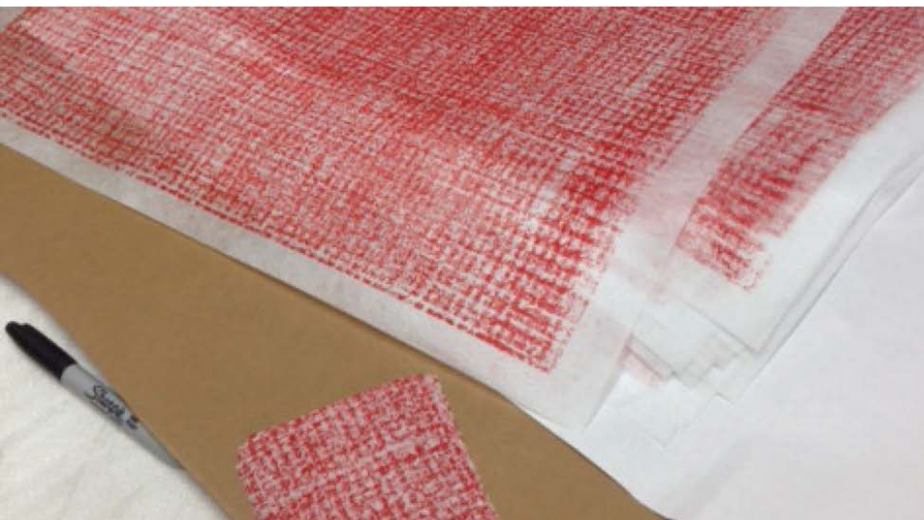
1" margin was required on each sheet to facilitate the silk screening process.
